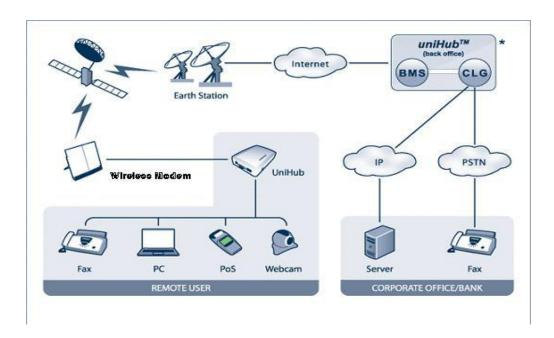
uniHub comes with several interface ports; the device simply need to be connected to the appropriate port and the uniHub configured using a web based interface.
